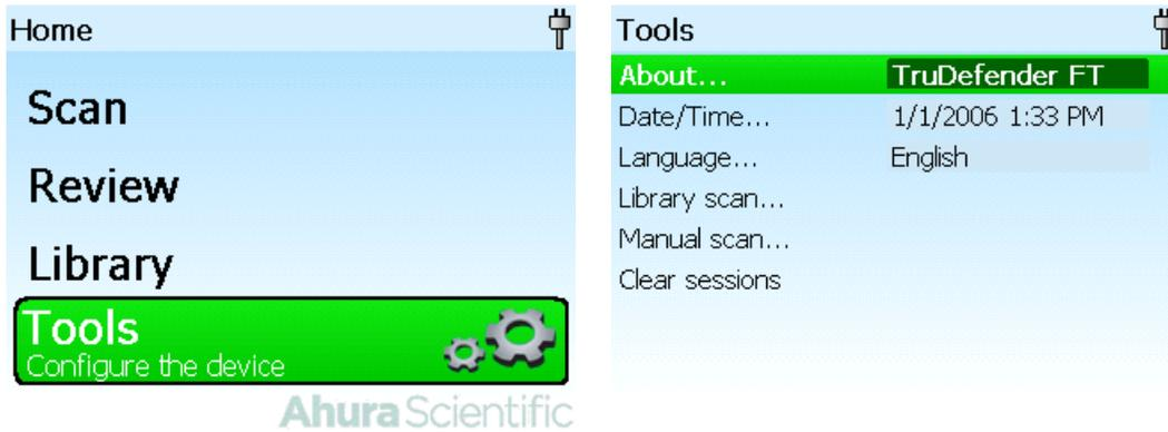
The Tools menu includes setting unit parameters, checking the revision level of the unit, clearing the sessions from memory, and other functions
