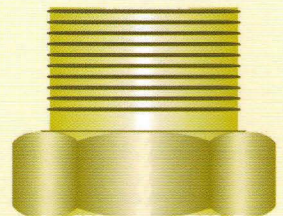
Straight (parallel) thread
